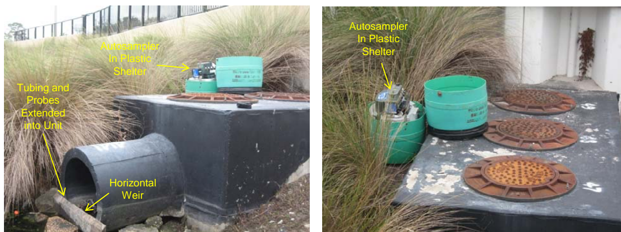
Figure 3-8. Photographs of Sampling Equipment Used at the Lake Concord Suntree Baffle Box Site.
