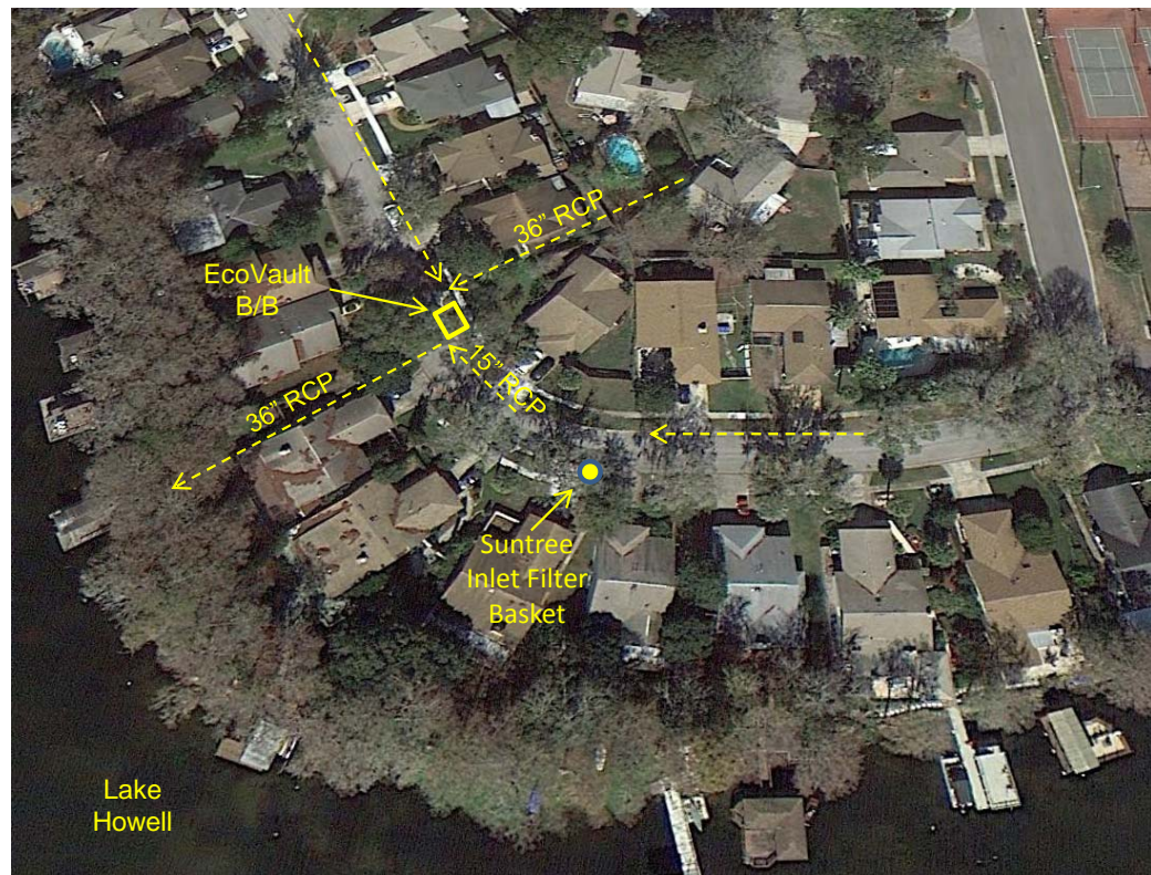
Figure 2-16. Drainage Patterns at the San Pablo Baffle Box Site.
