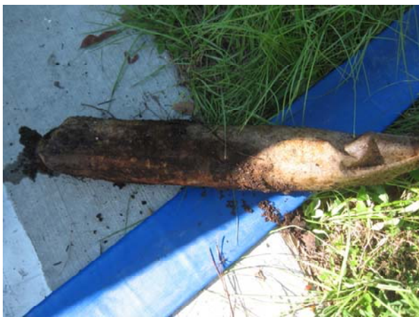
a. Exhausted Vault-Ox® insert removed from canister
