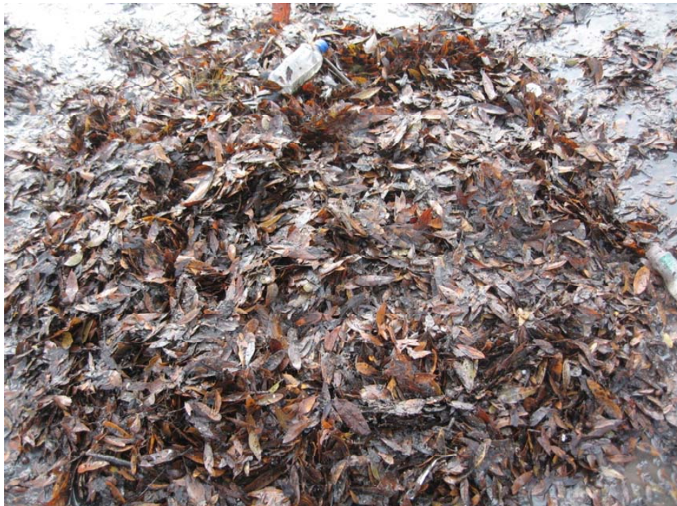
Figure 3-17. Photograph of Solids Removed from the CDS Unit.
