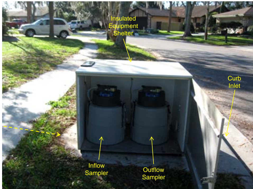
Figure 3-5. Photograph of Sampling Equipment Used at the San Pablo Avenue EcoVault® Site.
