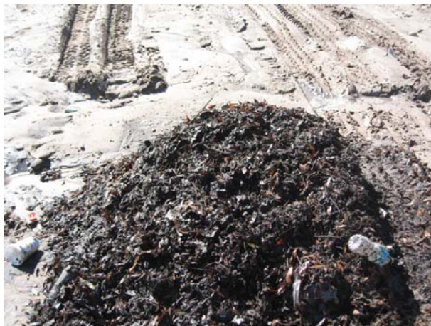
d. Material removed from the Lake Concord baffle box
