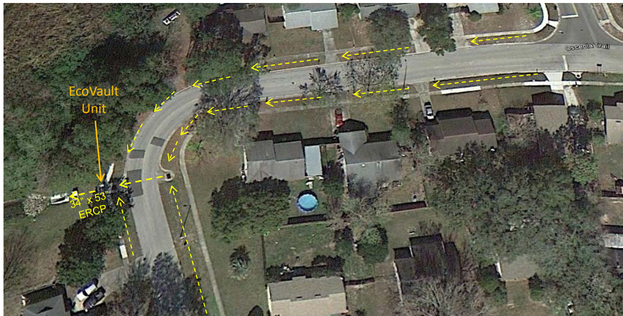
Figure 2-8. Drainage Patterns in the Vicinity of the Lake Hodge Baffle Box Site.
