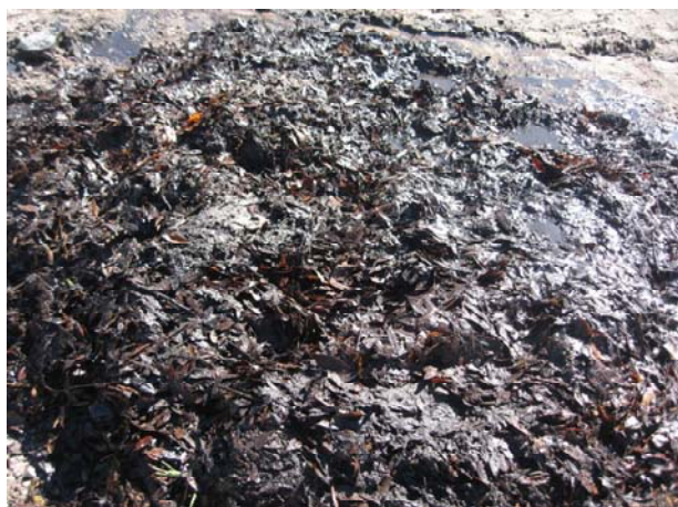
c. Material removed from the San Pablo baffle box
