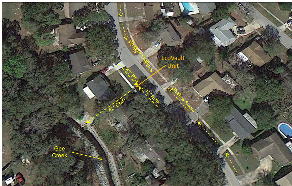
Figure 2-11. Drainage Patterns in the Vicinity of the Gee Creek Baffle Box Site.
